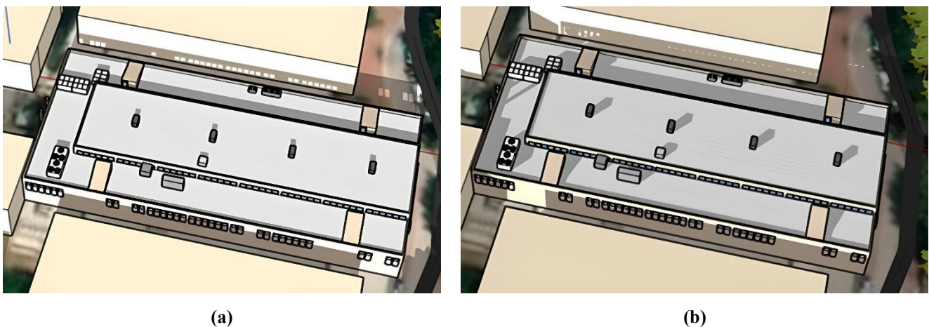
Figure 4 Shadows’ projection on the roof of the university building at (a) 12:00 and (b) 15:00.
