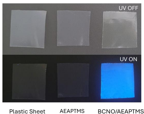
Figure 2. Image of plastic sheets covered either with siloxane matrix AEAPTMS or the combination AEAPTMS/BCNO either in dark or illumination with low intensity UV black light (max. at 365nm).
